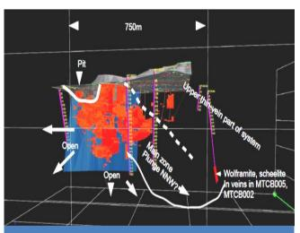
Figure 1. Cross section of the ore body at Mt Carbine looking west, showing mineralisation >0.22% tungsten and areas where the ore body is open to further exploration.
