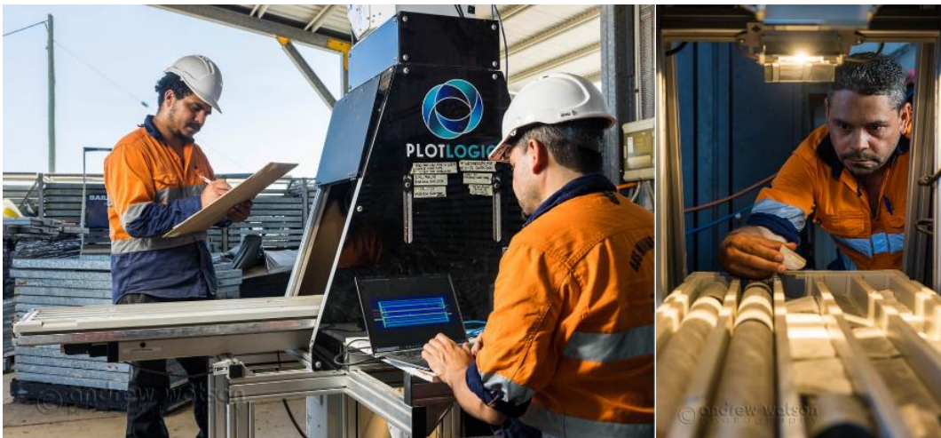
Figure 14 - Plotlogic's technology informs decision making through core sample scanning
