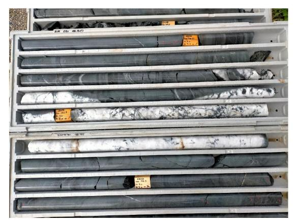
Figure 18 - Drill Core: High-grade wolframite-scheelite mineralisation from Hole EQ031 (showing intercept of 2.82m @ 1.81% WO<sub>3</sub>).
