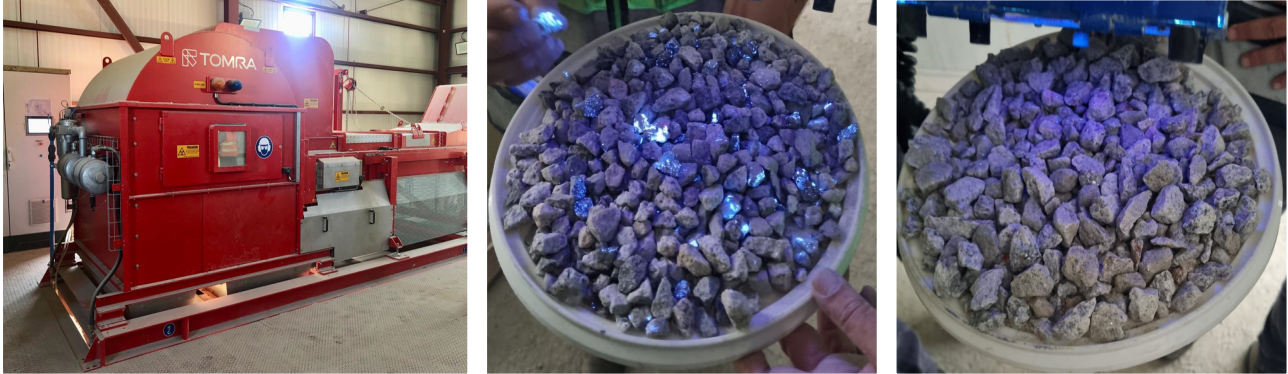
Fig.1 - Barruecopardo's first TOMRA XRT Ore Sorter (left); Shown under UV light are the sorter product from initial trials (center) and sorter waste (right)
