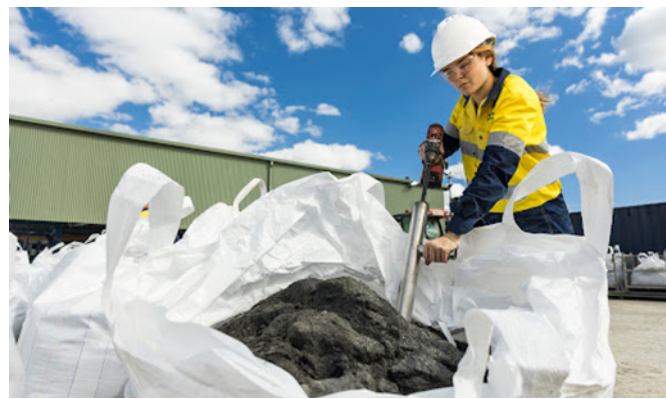
Fig.2 - Mt Carbine concentrate, sampling process (concentrate shipped with 50-55% WO 3 grade)
