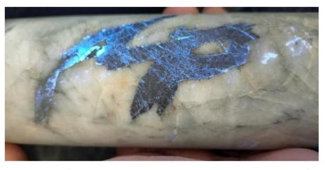
Example of scheelite mineralization overprinting wolframite
