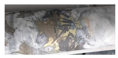
Intergrowth of wolframite and chalcopyrite in broad mineralized zone (EQ026, 93.2ms)
