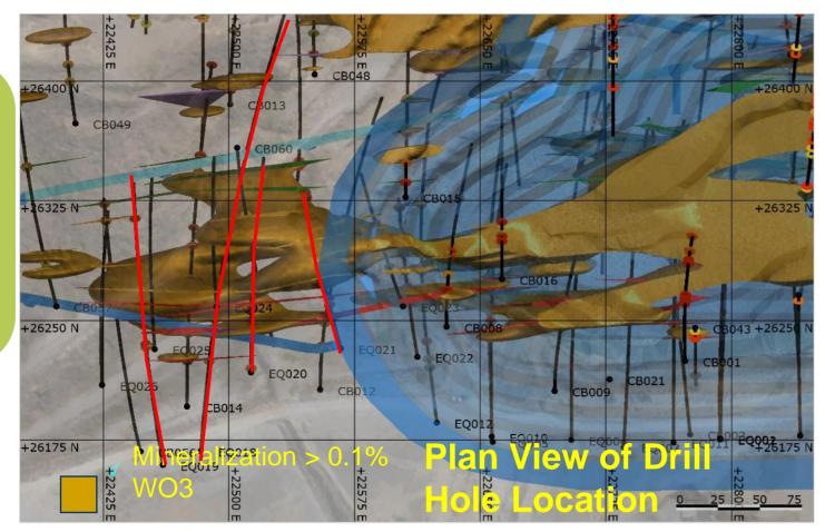
**Golden Colour** - Zone of + 0.1% WO3 Mineralization highlighting the western extension to the open pit mineralization.
