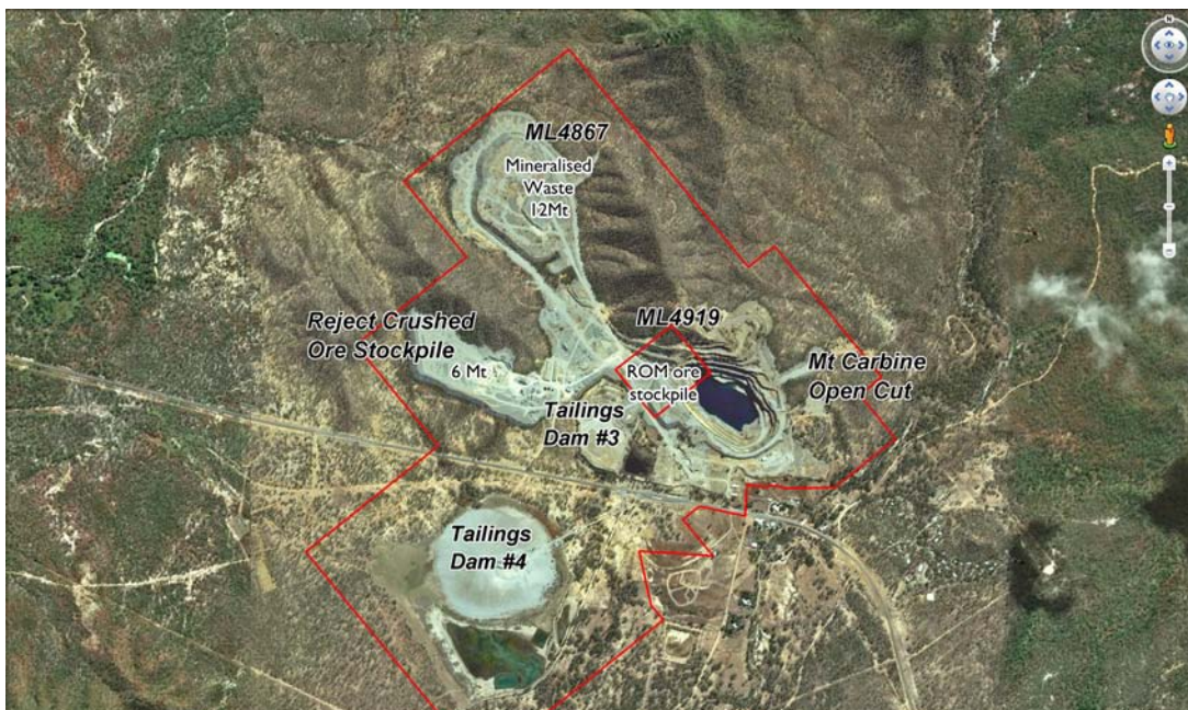
Figure 3. Aerial view of ML 4867 showing the location of the low grade stockpiles (mineralised waste, ore sorter reject and ROM stockpiles)
