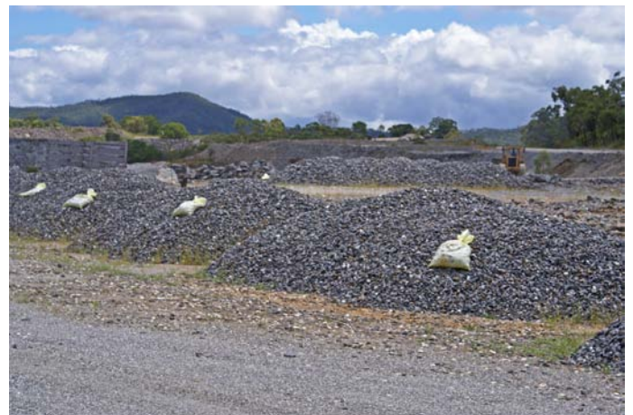
Daily production samples from the ore sorter results in mounds of reject material. Each days testwork was kept discrete.
