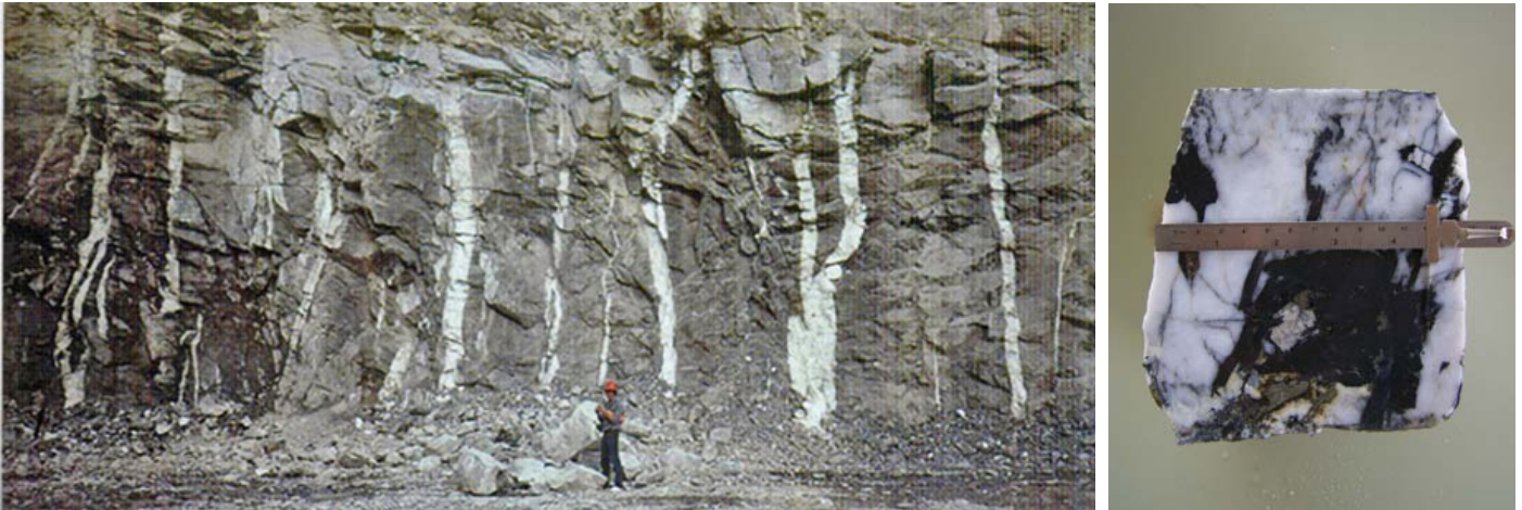
Figure 2. Quartz-wolframite sheeted quartz veining (white) separated by mostly barren host rock (dark gray) extending into the floor and north wall of the existing open cut. At right, photo of wolframite (black) in quartz vein.
