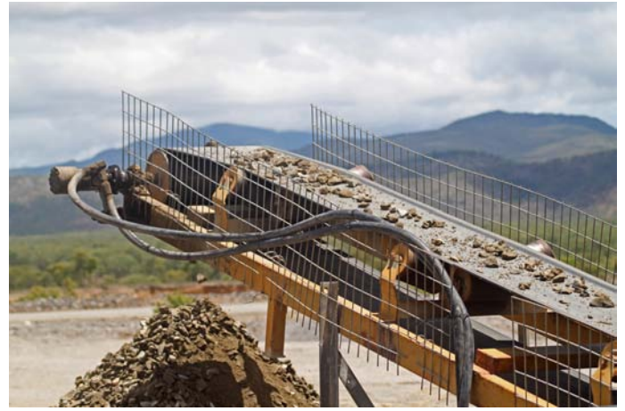
The ore sorter in action - the rejects conveyor with reject material from the sample stockpile.
