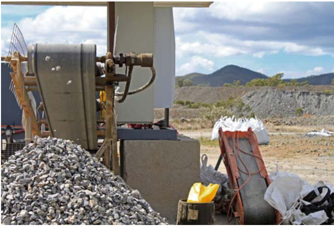
Ore sorter rejects conveyor behind reject material from the low grade stockpile.
