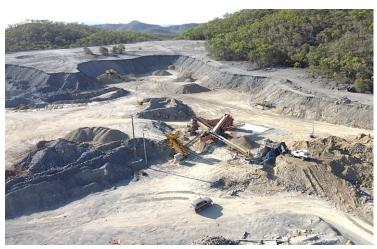
Pic.1 – Drone picture of Crushing & Screening Circuit of Quarry located next to historic mine waste dump
