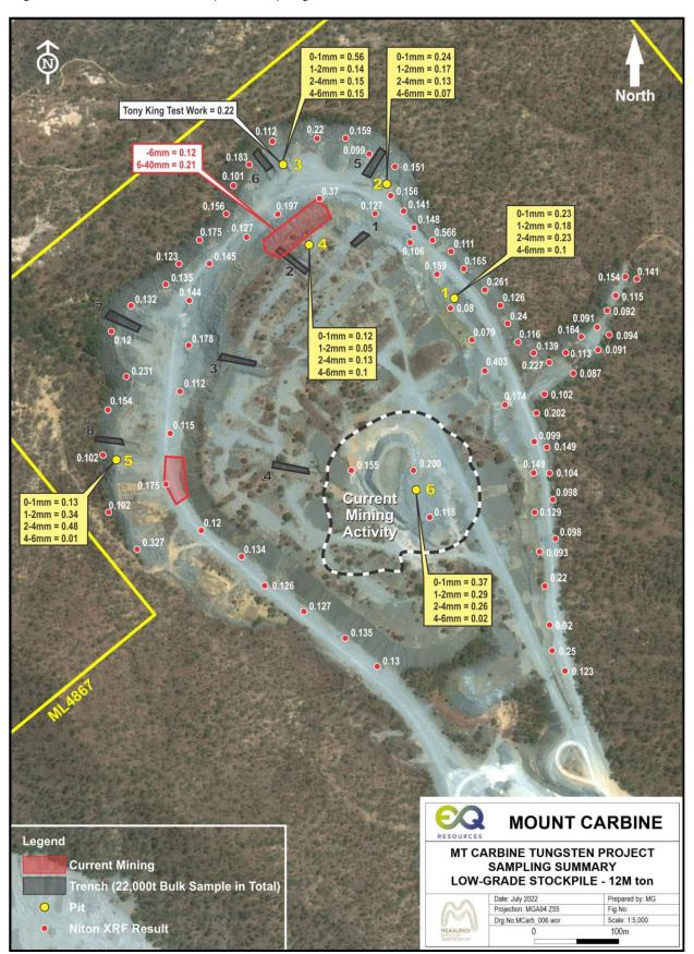
Figure 8-1: Low-Grade Stockpile Sampling Locations
