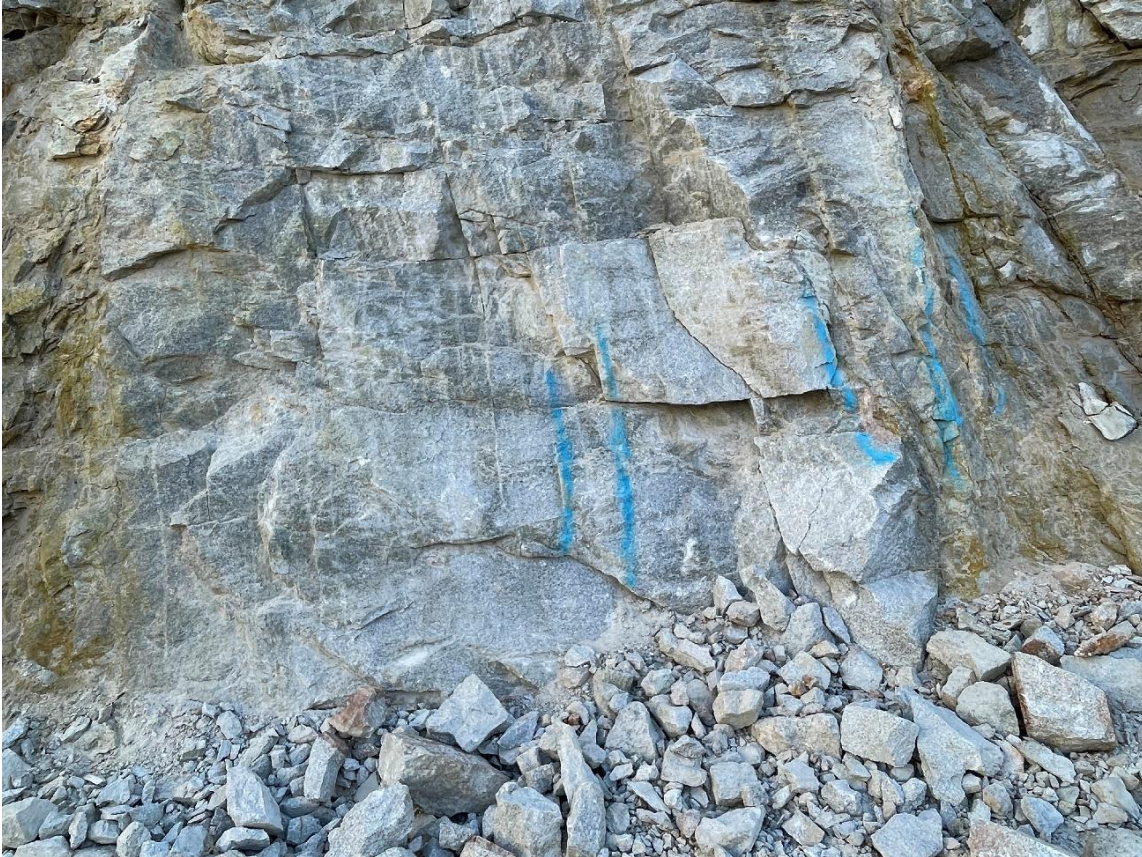
Figure 7-4 Vein swarm within the open pit. Veins marked in blue are mineralised. Dimension from left to right: 3m
