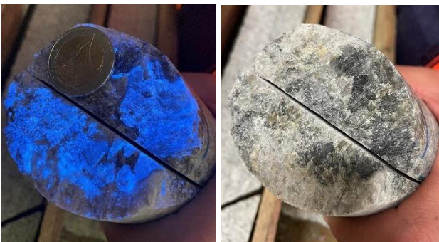
Figure 11-1 Example scheelite distribution on half core using UV light
