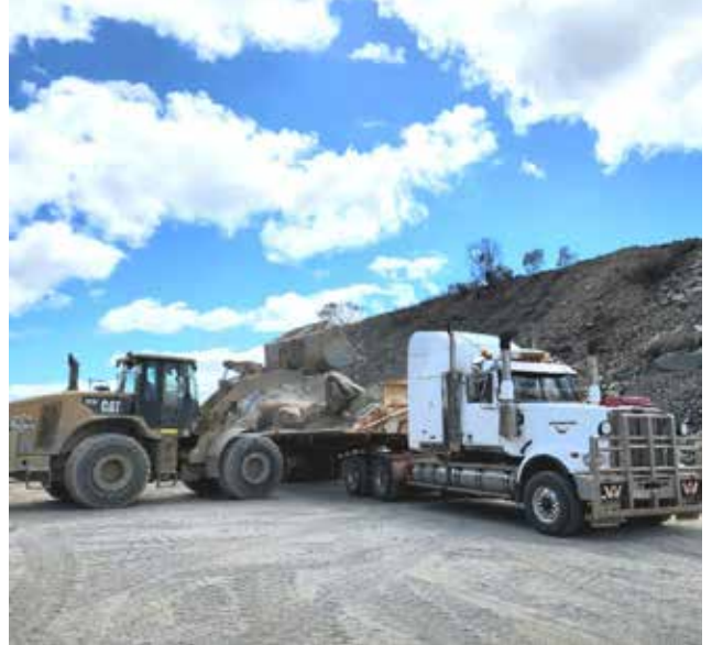
Large Rocks are used in the construction of breakwaters for local marinas.
