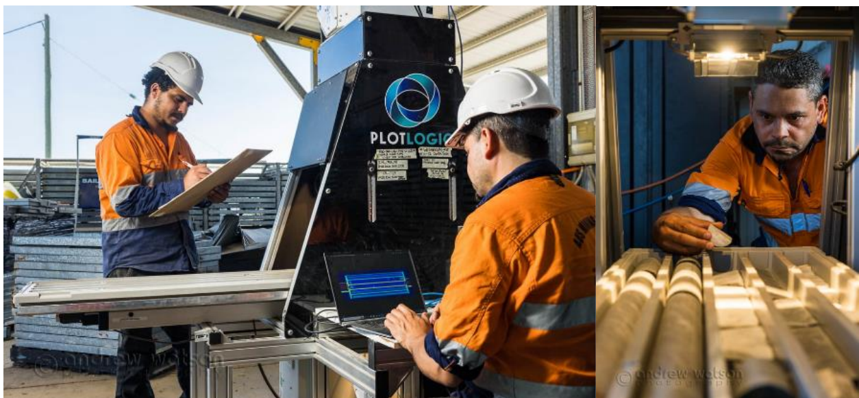
Figure 18 - Plotlogic's technology informs decision making through core sample scanning
