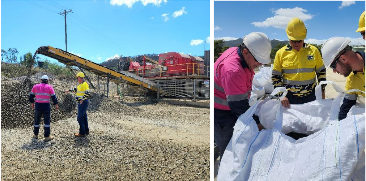
Figure 9 - Hon Scott Stewart MP witnesses the benefit of having two TOMRA XRT Ore Sorters installed on-site (left); Increased plant throughput leading to increased production of tungsten concentrate (right)
