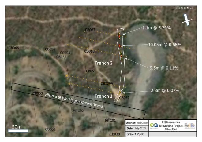
Fig.2 - Location of the two trenches and summary of results (grade shown in  $\%\ WO_3)$
