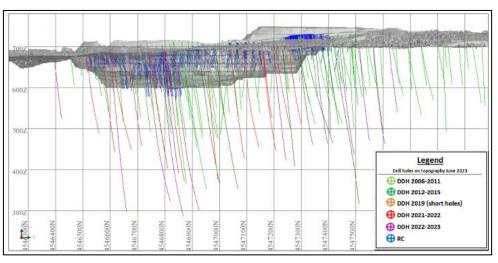
Fig. 2 - Long section of the deposit (North on left) showing topography, the pit and drill holes.
