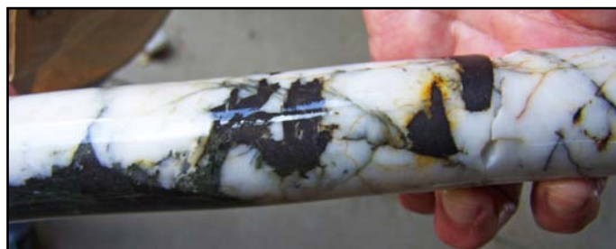
Above: Legacy core showing high-grade quartz-wolframite veining intersected to the NW of the existing open cut.
