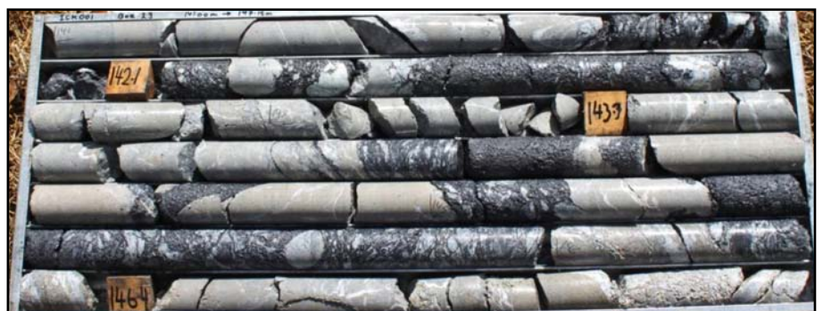
Highly altered / mineralised dyke (above left) and graphite (right) breccia zones within the 8m zone from 140m depth in drillhole ICK-001 grading 1.27g/t gold (above), and adjacent listwanite alteration at Peel Fault.
