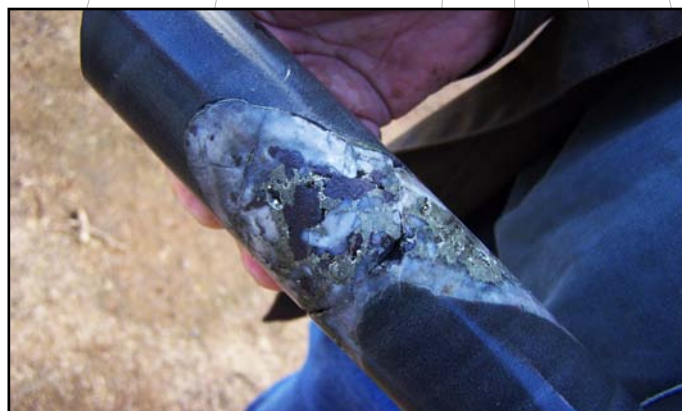
Above: Drill core at Tara showing Polymetallic sulphide vein.
