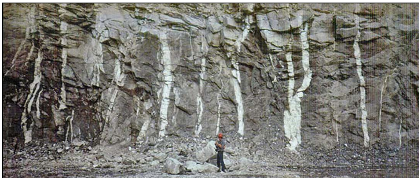
Above: Quartz-wolframite sheeted veining extending into the floor and north wall of the existing open cut. Photo circa 1986.
