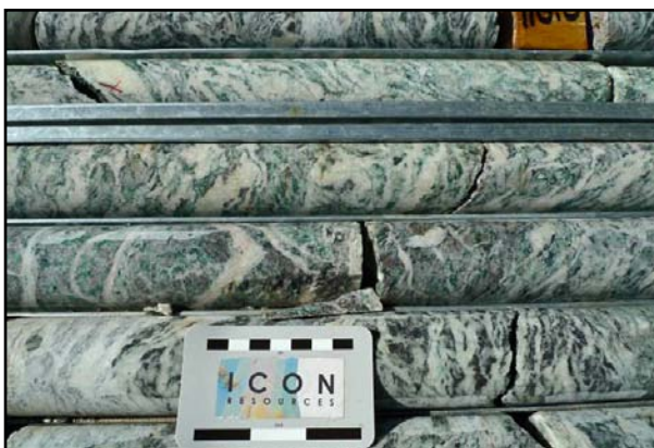
Highly altered / mineralised dyke (above left) and graphite (right) breccia zones within the 8m zone from 140m depth in drillhole ICK-001 grading 1.27g/t gold (above), and adjacent listwanite alteration at Peel Fault.
