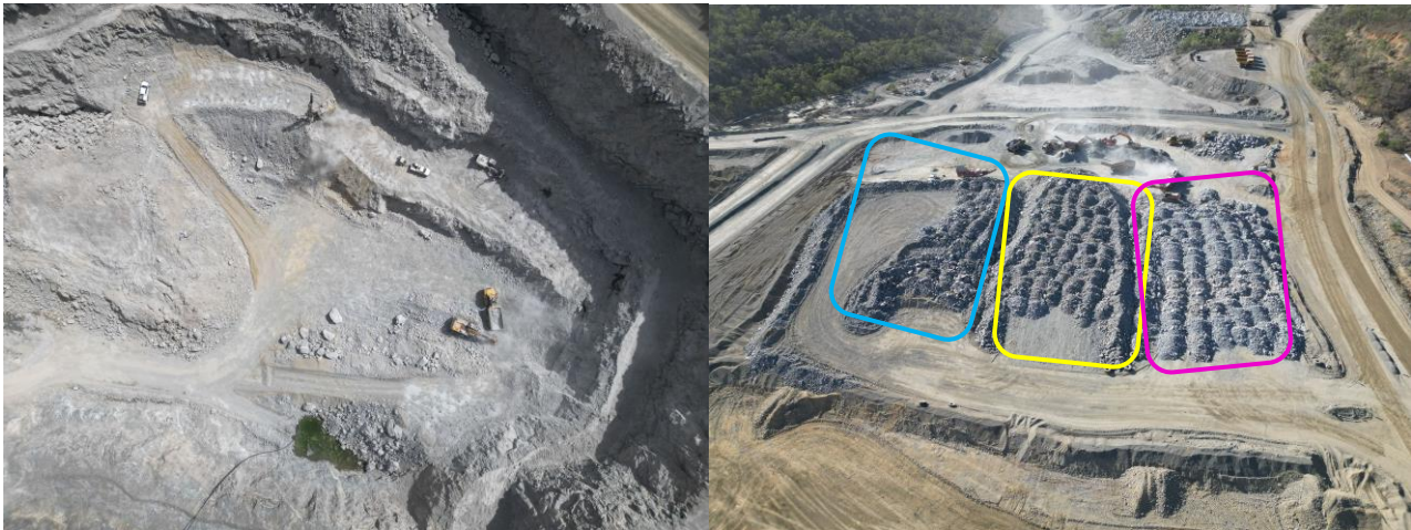
Excavation operations ongoing at the bottom of the pit (Left); Current stockpiles, sorted by grade from left to right: Blue 'low grade', Yellow 'medium grade', Pink 'high grade' (Right)
