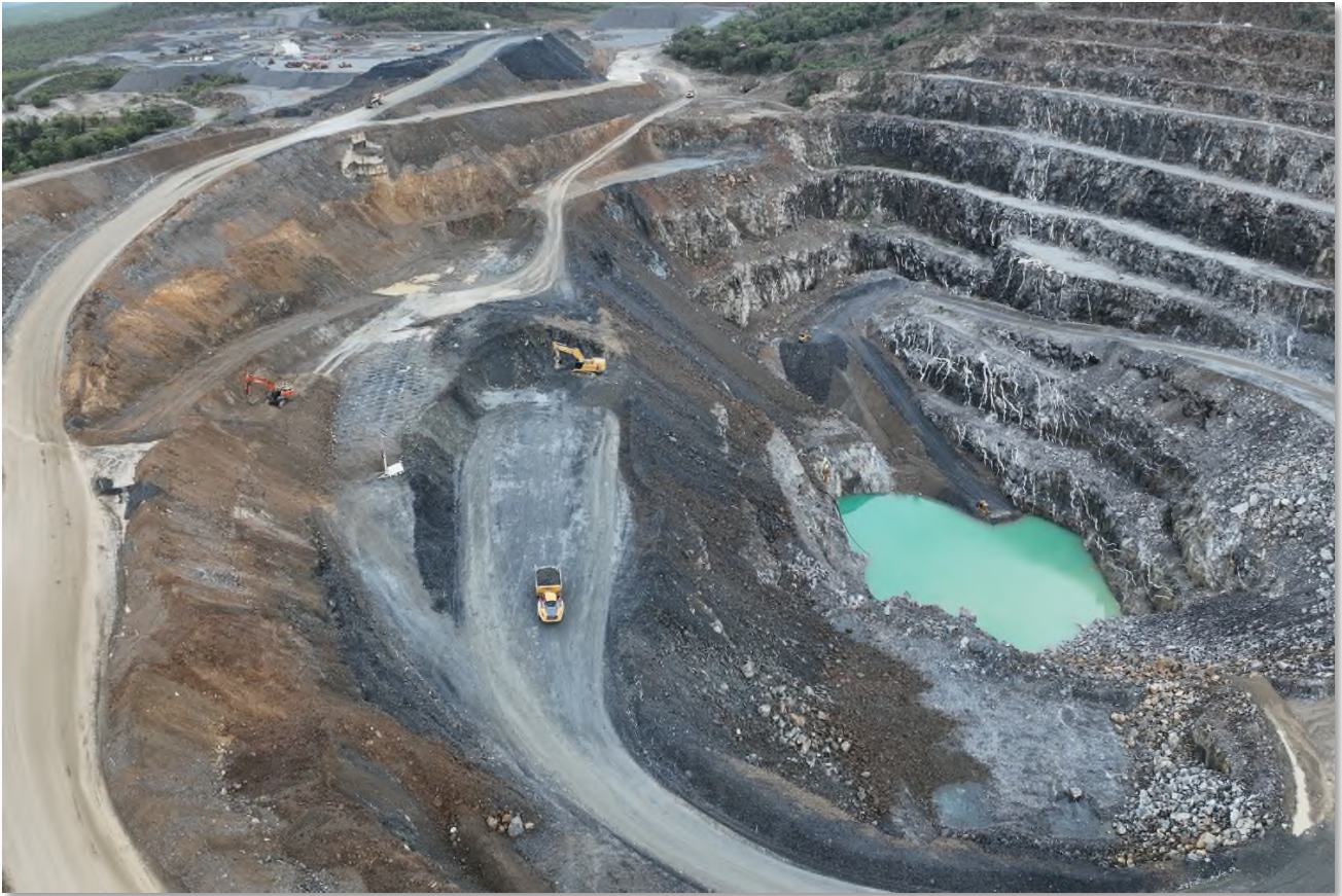
Above: Mining operations advancing on the South Wall, with drilled blast holes on the 345-335 RL level
