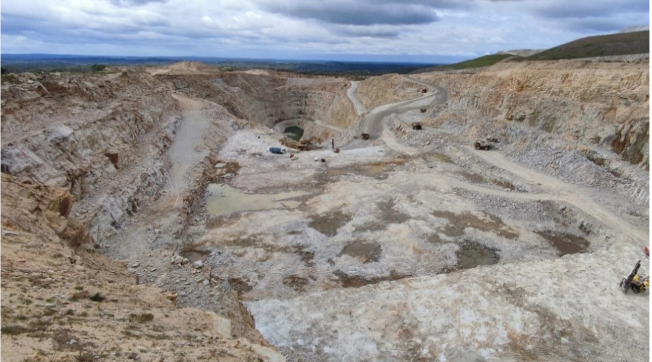
Northern area of Phase 6 at elevation 670 RL, including the access ramp and first blasts in the 660 RL bench.
