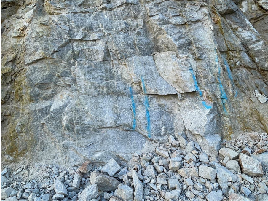
Figure 4-4 Vein swarm within the open pit. Veins marked in blue are mineralised. Dimension from left to right: 3m
