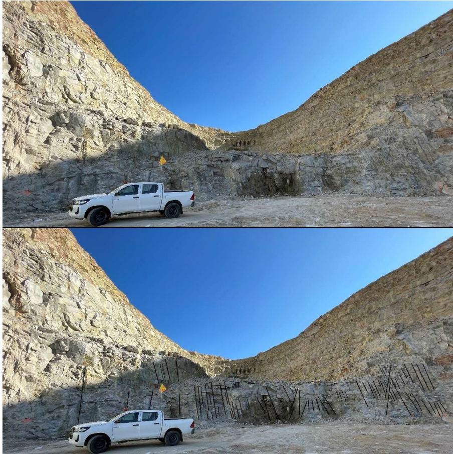
Figure 4-5 Barruecopardo northern pit wall with subvertical vein swarms and/or fractures (lower picture interpreted)
