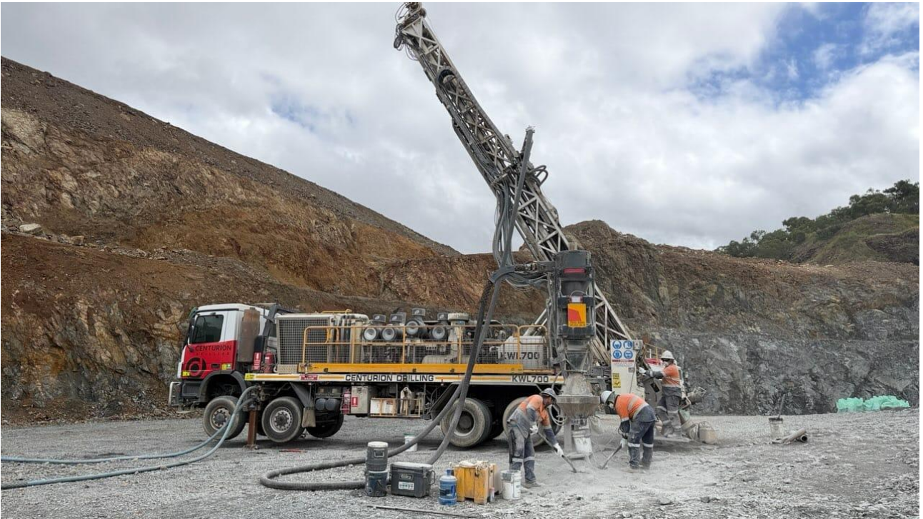
Figure 1: RC drill rig on site at Mt Carbine Tungsten Mine
