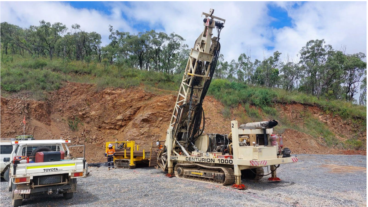
Figure 2: Diamond drill rig on site at Mt Carbine Tungsten Mine
