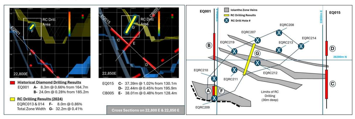
Infill RC Drilling at 10m spacing into the Iolanthe Vein System, confirming consistency of high-grade sections. Individual veins ranging with true widths of 0.3-2.5m were intersected at 0.5% to 3.66% WO<sub>3</sub> grades. Interpretation confirms veins are increasing in grade as Stage 2 Pit commences at the 325m level. Drilling into the Iolanthe Vein System, considered the strongest zone identified so far in the open pit, does not reflect the entire system but rather 1 of 4 major vein packages.
