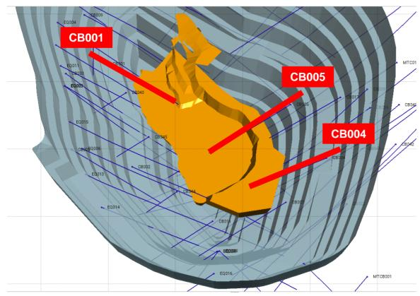
Fig.1 - Top view of 'Phase 1 Pit' (Aug'23 - July'24), target ore in orange; 3 historical (pre-EQR times) in blue, CB001 was misplaced in survey
