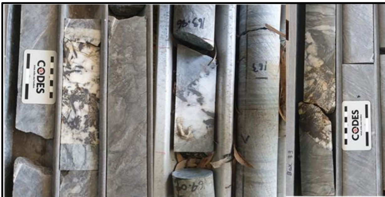
Figure 9: King Veins Showing Coarse Vein Textures of Wolframite Crystals
