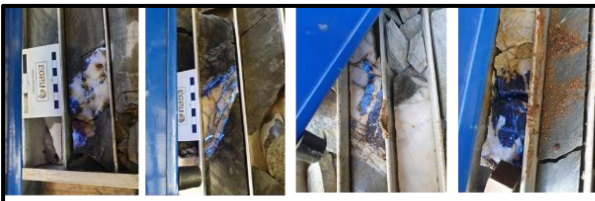
Figure 10: Core Showing Late Replacement of Wolframite by Fine Network Retrograde Scheelite
