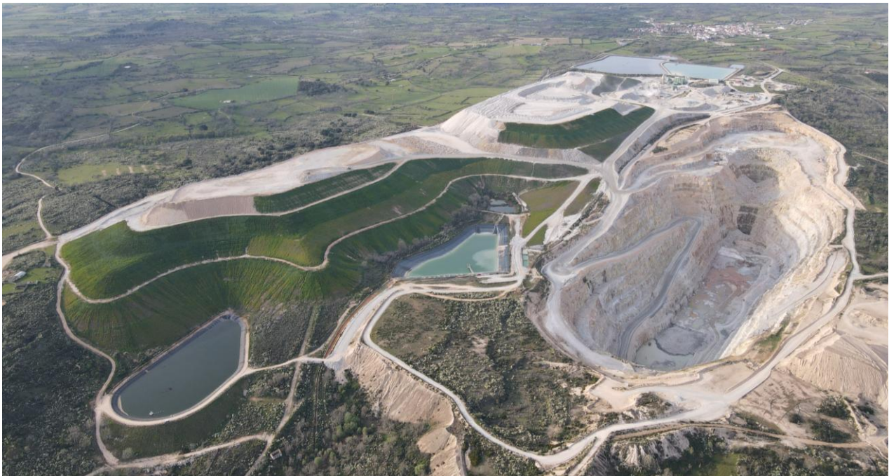
Picture above: The Barruecopardo Mine Open Pit as at March 2025 looking north, with ongoing progressive rehabilitation of the waste dumps near the water dams on the front left.
