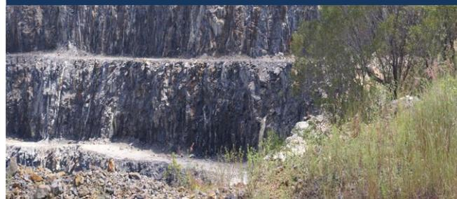
Mt Carbine Tungsten Deposit – vertical, sub-parallel, quartz Veins hosting wolframite and scheelite mineralization.
