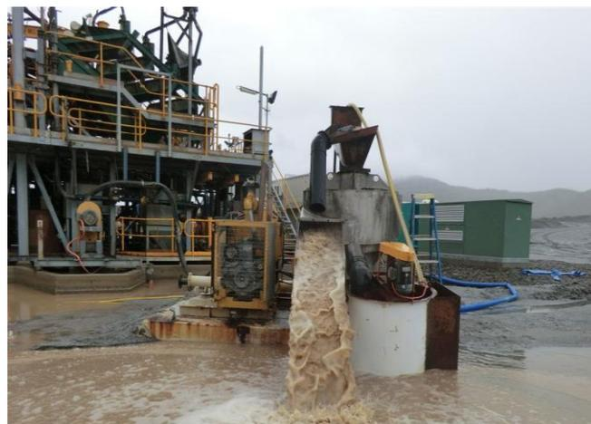
Testing of Ultra Fines Centrifuge recovering tungsten particles down to three micron.
