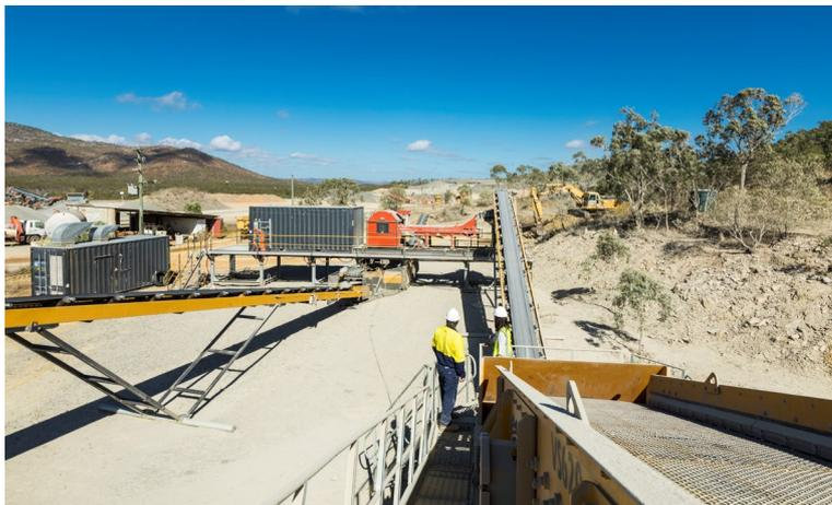
Figure 2 - XRT Sorter Pilot Plant
