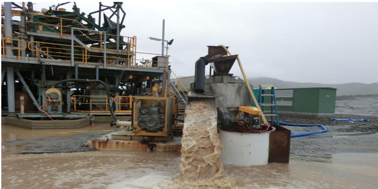
Testing of Ultra Fines Centrifuge recovering tungsten particles down to three micron.
