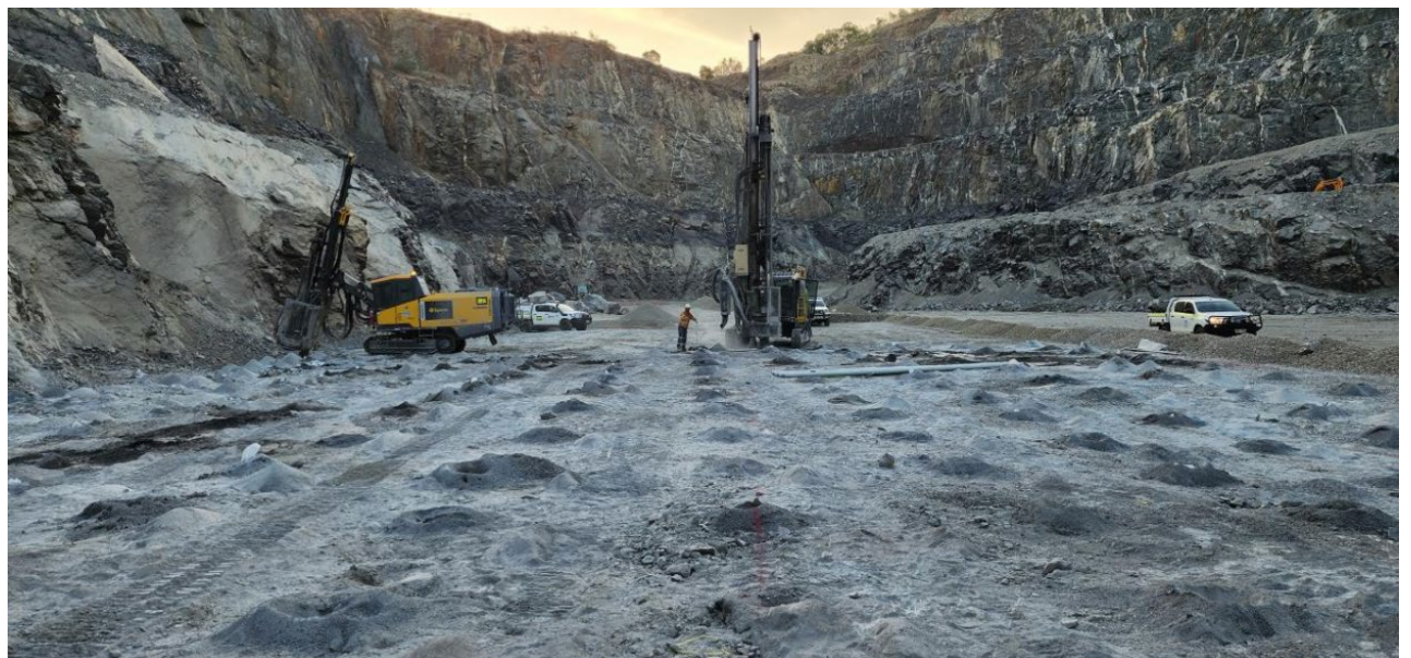
Figure 5: Orana Drill and Blast Rigs
