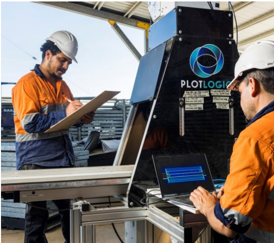
Figure 12: Plot Logic sensor, scanning drill core.
