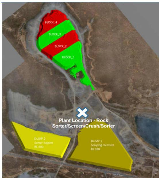
Figure 2 - Site layout (stockpile mining plan)
