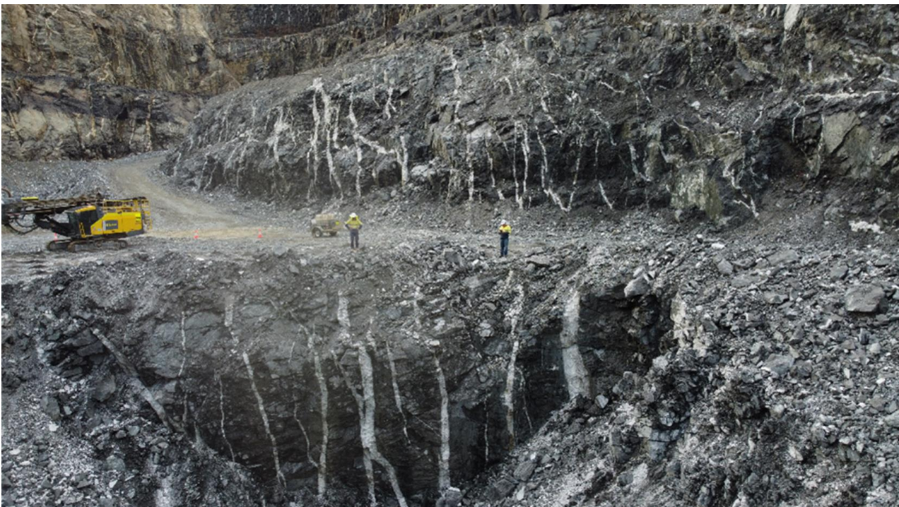
Johnson veins showing up in the pit – looking at blast 305-002 wall. Individual veins grade looks high by visual inspection with the entire face being 0.28% in this region. Drill rig on the left during RC Control drilling.
