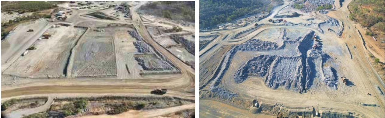
ROM 1 Stockpile in the first week of Open Cut Mining (Left); ROM 1 Stockpiles end of December 2023 (Right)
