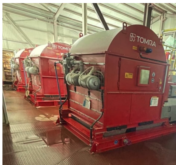
Fig.1 – Saloro XRT Ore Sorters in operation
