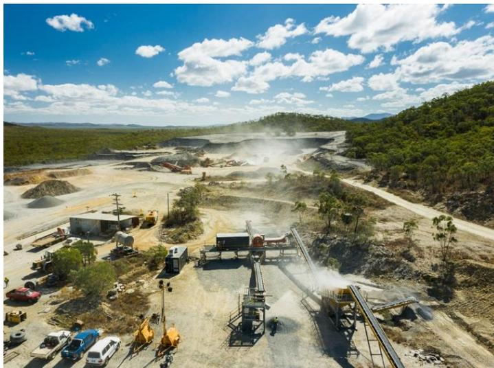
**Figure 1 – XRT Sorter Pilot Plant**
