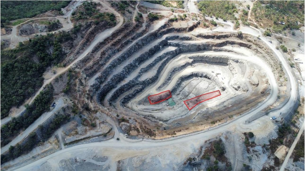
Figure 3 - The dewatered Andy White Open Pit is undergoing final preparations before mining recommences later this month. Red Blocks indicate 1st Month mining areas.
