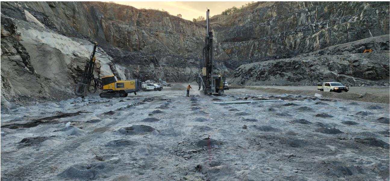
Figure 1 - Orana Drilling Blast Holes
