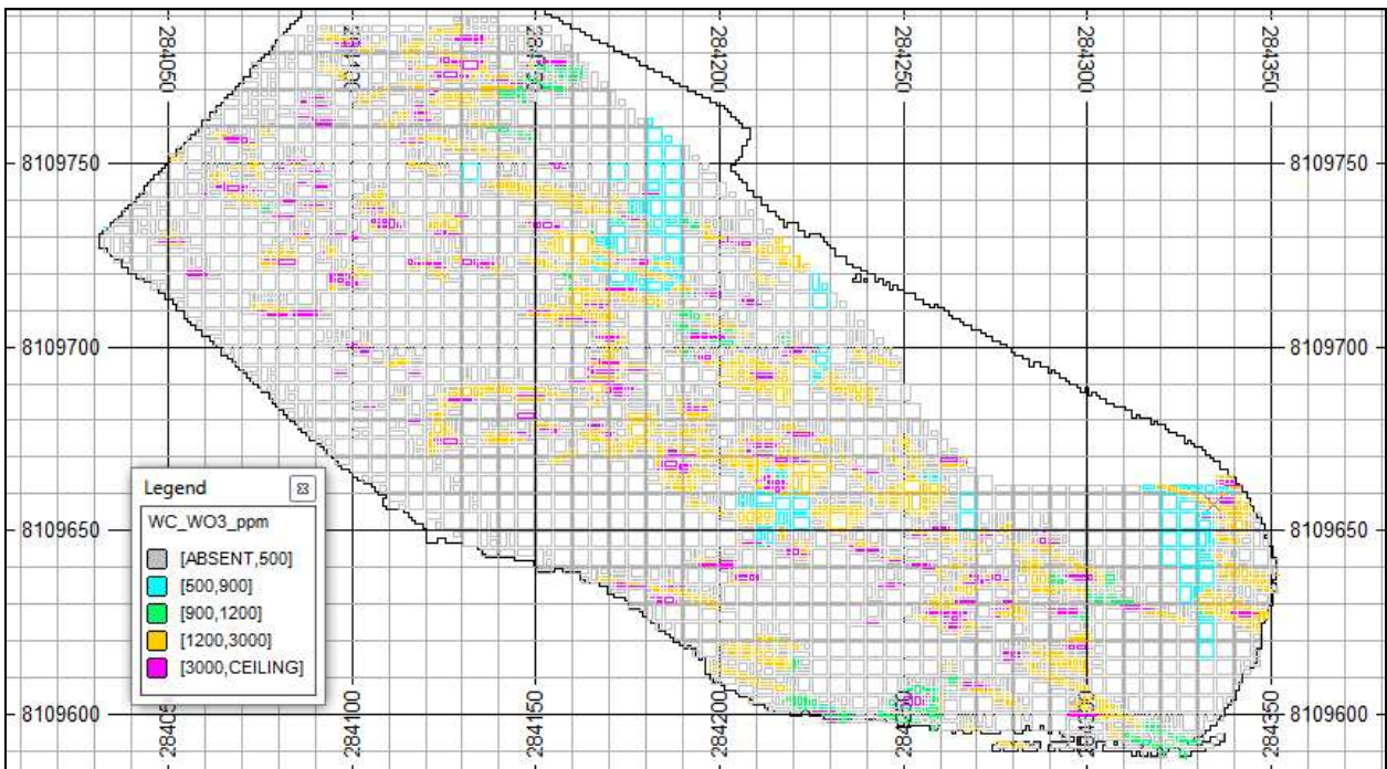
Figure 14-16. Plan at 573.25mRL - Test Evaluation Model, March 13- March 14 (Based only on DD and RC data)
