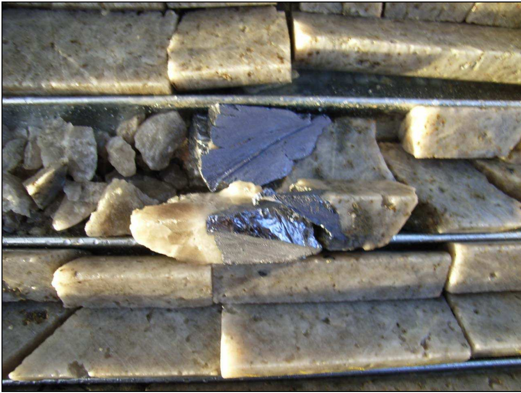
Figure 6-1. High Grade Molybdenite Intersection (typical of those requiring hand picking during analysis)
