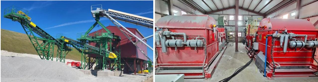
Fig.4 - Saloro's XRT Sorting Plant fully commissioned; 2x Tomra XRT Sorters (COM Tertiary XRT 1200)
