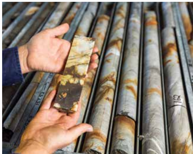
Drill core with wolframite mineralisation
