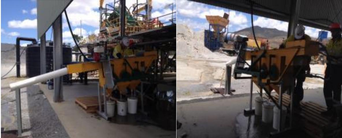
**Jig test-work being carried out at the Tailings Retreatment operation.**
