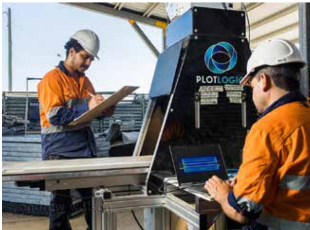
Plotlogic sensor, scanning drill core.
