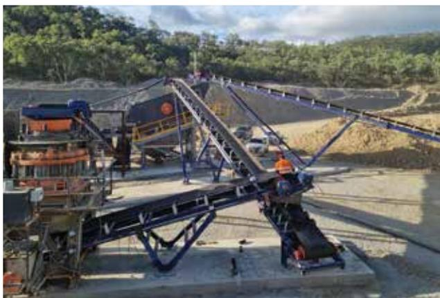
Crushing and Screening Plant with the Cone Crusher at the forefront.
