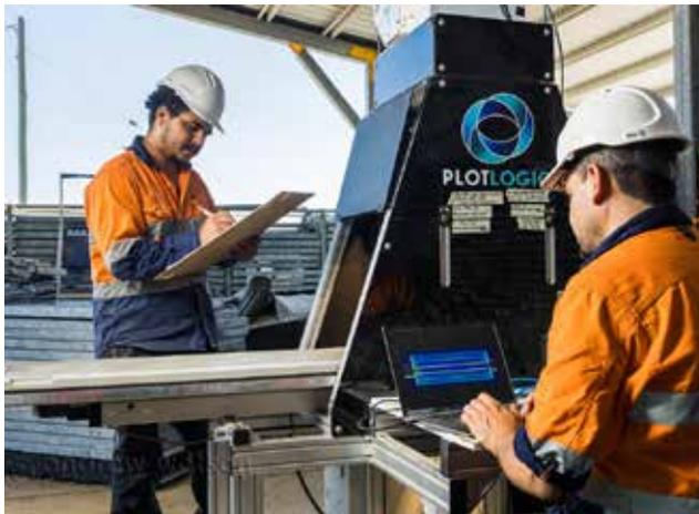
Plotlogic sensor, scanning drill core.
