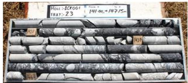
**Interval assaying 8m at 1.27g/t Au from 140m in hole ICK001, showing carbonaceous gouge (dark grey) intruded by altered quartz monzodiorite dykes (light grey). It is now thought that most of the gold in this interval is in the carbonaceous gouge and this will be confirmed by further sampling.**
