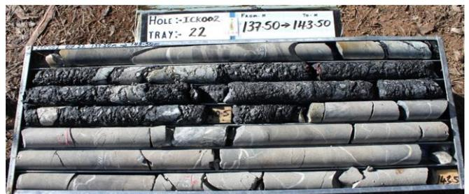
**Interval assaying 3.69g/t Au from 138.5m to 140.65m in the dark grey/black carbonaceous fault gouge adjacent to altered monzodiorite in Icon drill hole ICK 002.**
