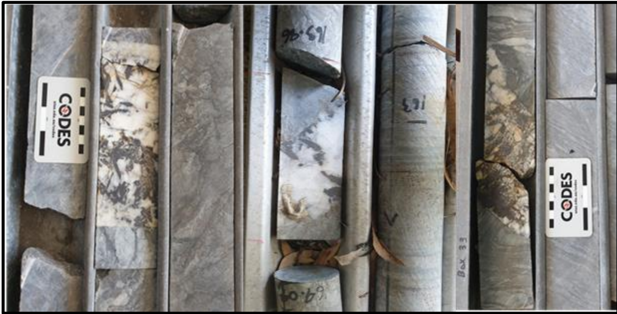
Figure 18: King Veins Showing Coarse Vein Textures of Wolframite Crystals
