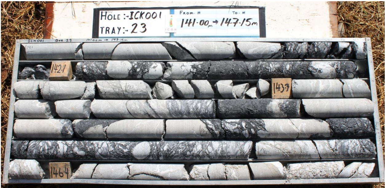
Interval assaying 8m at 1.27g/t Au from 140m in hole ICK001, showing carbonaceous gouge (dark grey) intruded by altered quartz monzodiorite dykes (light grey). It is now thought that most of the gold in this interval is in the carbonaceous gouge and this will be confirmed by further sampling.
