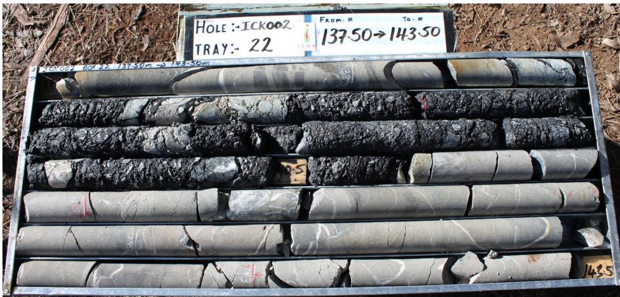
Interval assaying 3.69g/t Au from 138.5m to 140.65m in the dark grey/black carbonaceous fault gouge adjacent to altered monzodiorite in Icon drill hole ICK 002.
