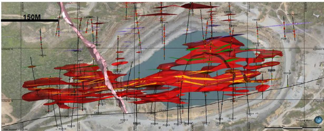
Figure 2 – Ore shapes with different grade mineralisation (green/yellow shapes highlighting ore blocks >0.20% WO<sub>3</sub>, red shapes highlighting ore blocks >0.05% WO<sub>3</sub>)
