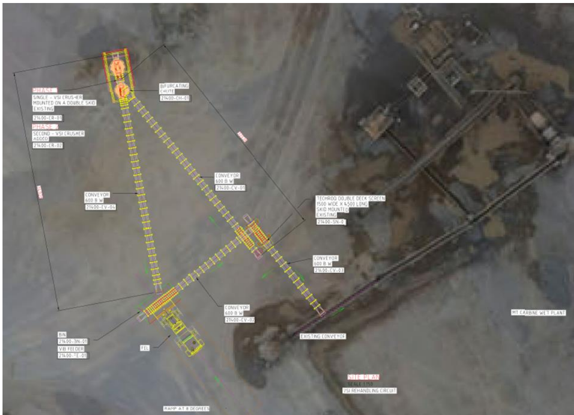
Figure 23: Phase 1 Rehandling Circuit
