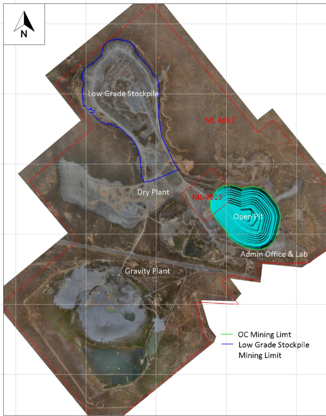
Figure 3: LGS & Open Pit locations relative to the Crushing and Screening Plant and Processing plant
