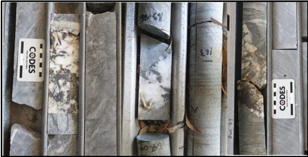
Figure 9: King Veins Showing Coarse Vein Textures of Wolframite Crystals
