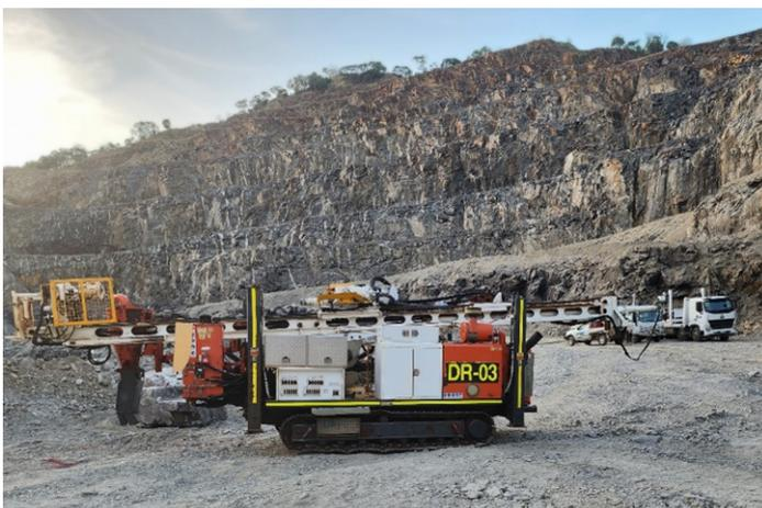
Fig. 2 - Grade control Drill Rig in the Mt Carbine Andy White Open Pit
