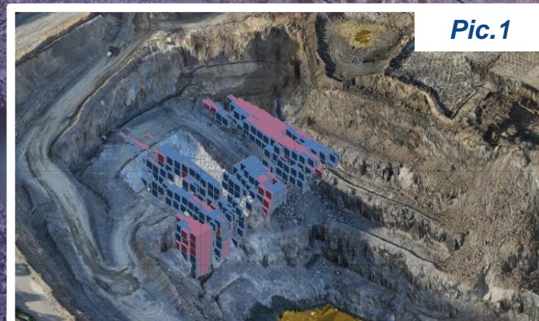
**Pic.1:** Resources Block Model showing an extract of the ore blocks in the ore body in the South-East (Section '0' and '8') below 335RL.
