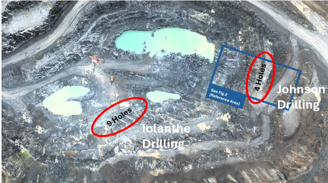
Fig.1 - Drone photo of pit after heavy rain when the veins are exposed; 13 RC holes drilled at 70 degrees and 33m length each
