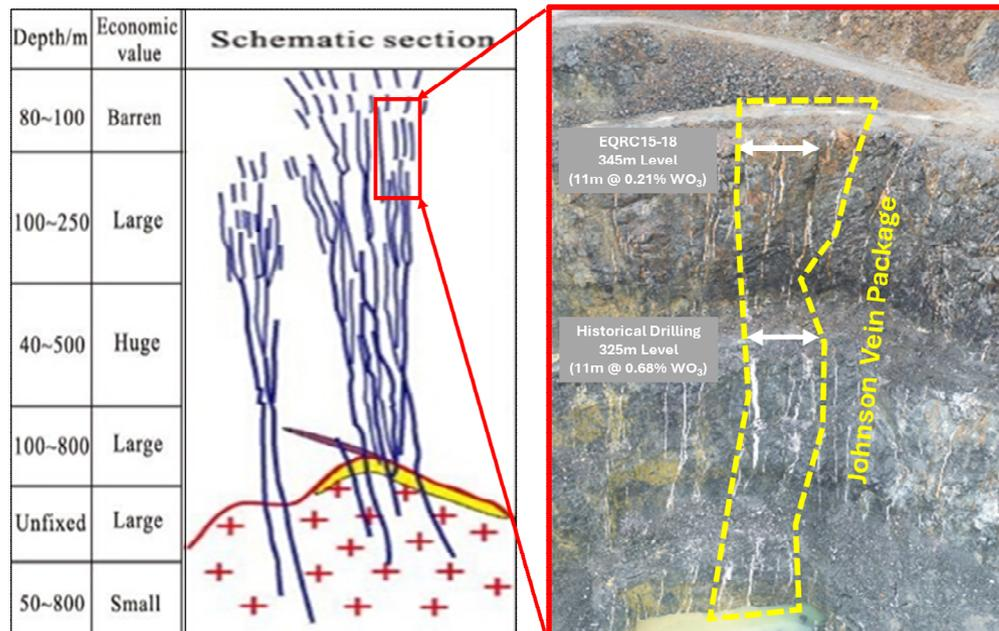
Fig.2 - Drill results and interpretation of Johnson Vein Package; Comparing with geological model for sheeted-vein tungsten deposits, left side (Source: Gu, J.Y., Morphological Zonation of Tungsten Deposits in South China)
