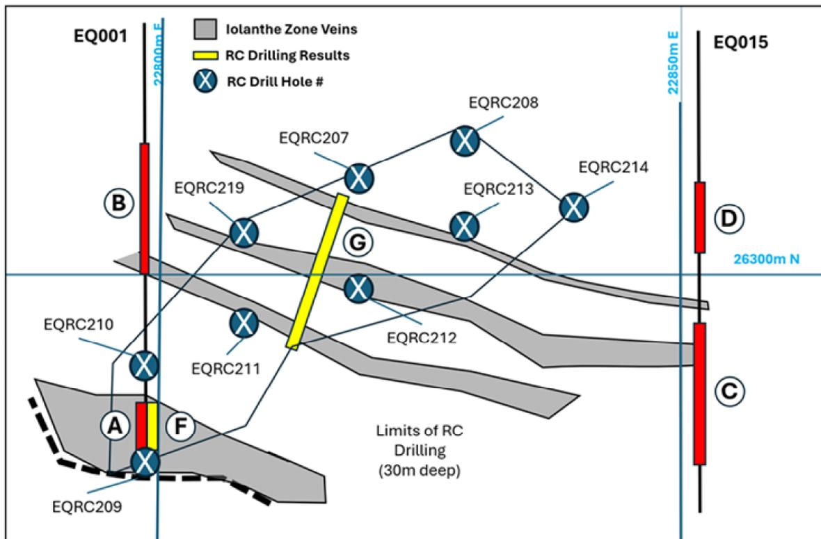
Fig.3 - Close up of RC drilling in Iolanthe Vein System showing 4 of the packages intercepted; the ore zone across these four veins in yellow is compared with historical EQR drilling on 50m centres in red
