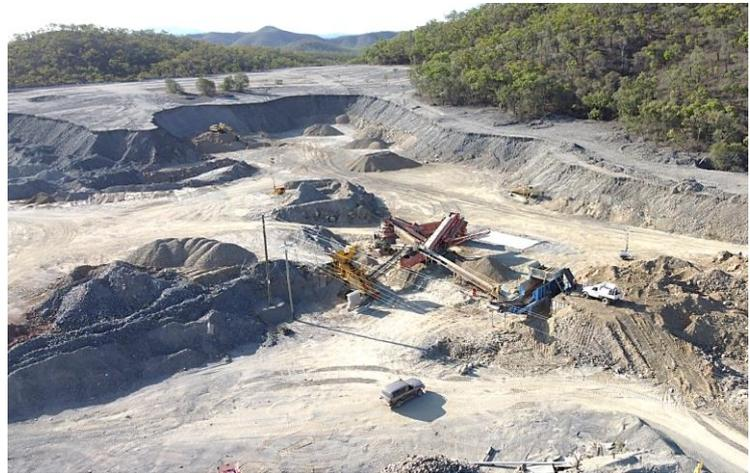
Pic.1 – Drone picture of Crushing & Screening Circuit of Quarry located next to historic mine waste dump
