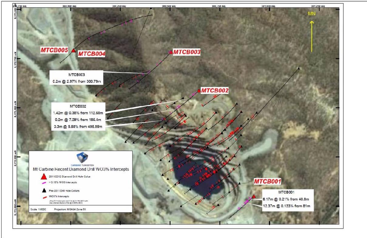
Plan view of drill holes used in resource estimation for the Mt Carbine tungsten deposit, plus a summary of results from exploration holes MTCB 001-005 drilled in 2012.
