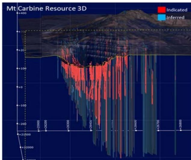
3D Block Model with Indicated & Inferred Resources cut thru at 22,900E
